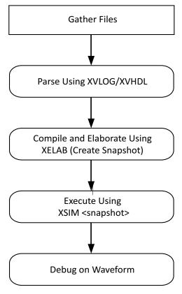
Figure 7-4: Behavioral Simulation Process
