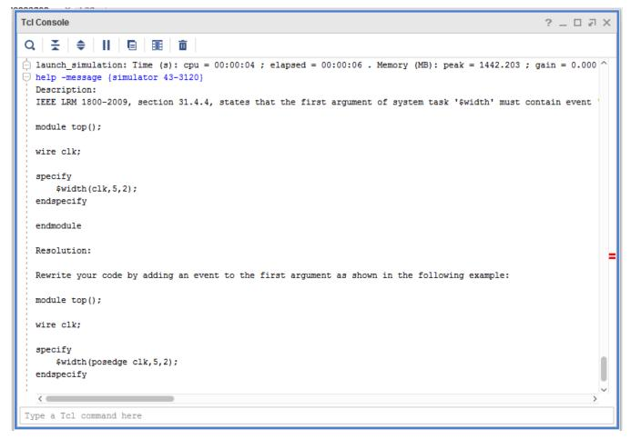
Figure 4-17: Simulator Message Description and Resolution Information
