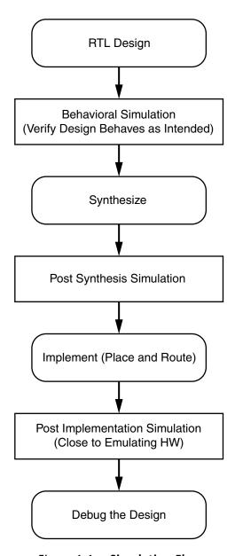
Figure 1-1: Simulation Flow
