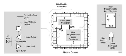
Figure E-1: Built-in FPGA Initialization Circuitry Diagram
