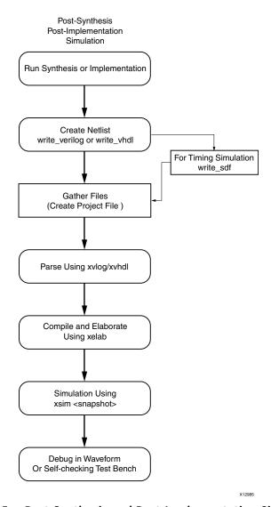
Figure 7-5: Post-Synthesis and Post-Implementation Simulation
