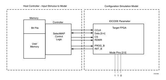
Figure E-2: Block Diagram of Model Interaction
