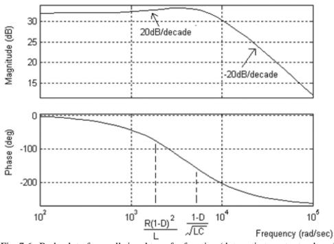
Fig. 7.6. Bode plot of a small signal transfer function (duty ratio to output voltage) of a boost converter in continuous mode
