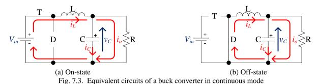
Equivalent circuits of a buck converter in on-state and off-state are shown in Fig. 7.3. T is the transistor and D is the free-wheel diode of the converter. State-space variable of the converter is taken as the set of the inductor current,  $i_L$ , and the output filtering capacitor voltage,  $v_C$  which is also the output voltage.  $i_o$  is the output current and is equal to  $v_C/R$ . *d* is the small-signal variation of the duty ratio of the gate signal.
