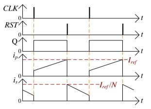
Fig. 7.12. Idealised waveforms of a current loop of a flyback converter with peak current mode control
