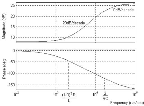
Fig. 7.13. Bode plot of a boost converter with inner current loop
