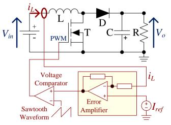
Fig. 7.10. An inner average current loop of a boost converter
