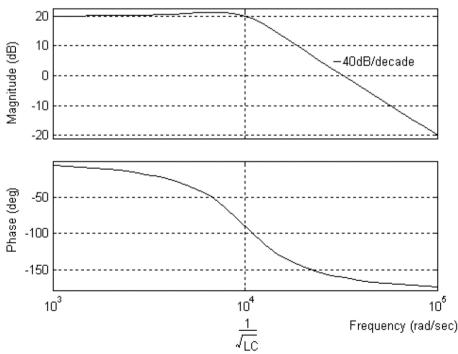
Fig. 7.4. Bode plot of a small signal transfer function (duty ratio to output voltage) of a buck converter in continuous mode
