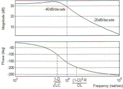
Fig. 7.8. Bode plot of a small signal transfer function (duty ratio to output voltage) of a buck-boost converter in continuous mode
