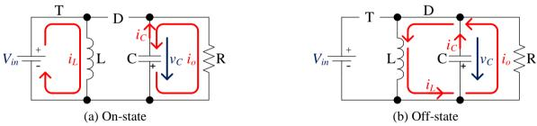
Fig. 7.7. Equivalent circuits of a buck-boost converter in continuous mode
